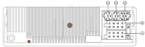
**Warning!** Terminal 30 and terminal 15 must always be connected separately, otherwise an excessive current consumption occurs when the unit is switched off. Connection socket A is not the same for all vehicle types. Therefore, always measure voltages before installation.
